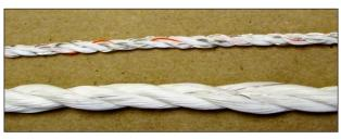
Figure 3. Two different styles of 9-stranded Polywire
