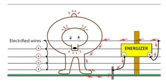
Figure 1. An all-hot electrified fence design. All wires are connected to each other in series and to the positive terminal on the energizer. The negative terminal of the energizer is connected to the grounding rod.
