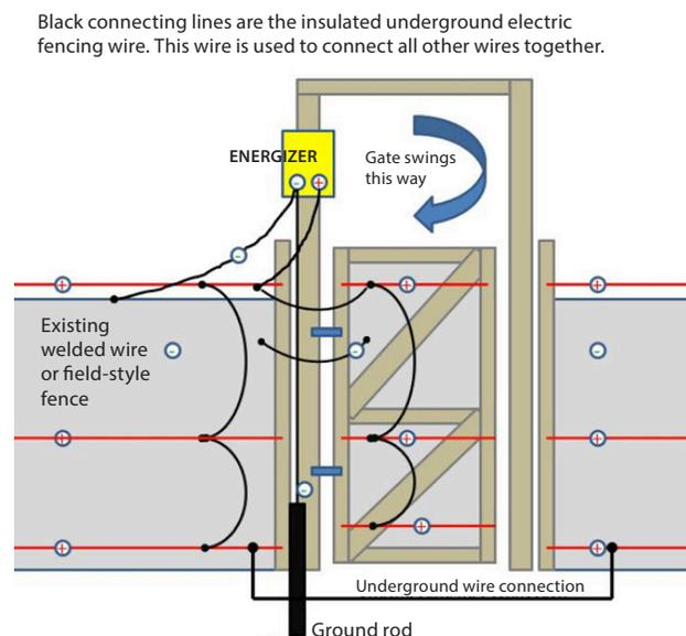
Figure 8. An example of how a gate can be electrified by attaching it to the electrified lines on the main fence, and how two sections of fence can be electrified with an underground wire connection.
