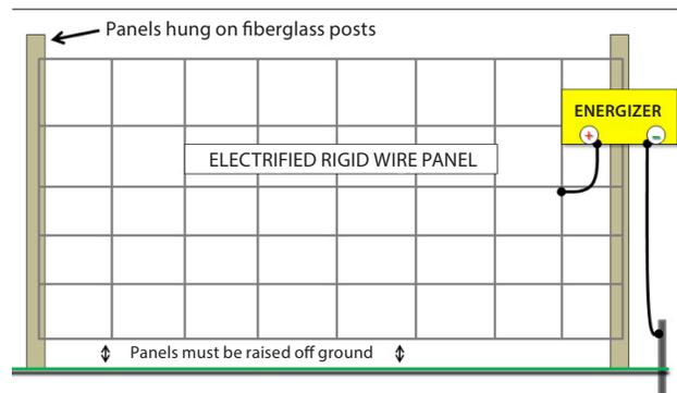
Figure 5. Electrified rigid wire panel. The panel is raised off the ground and insulated by hanging it from fiberglass posts. The wire panel is electrified by connecting it directly to the positive terminal on the energizer. The ground rod is connected to the negative terminal of the energizer.
