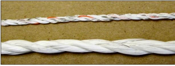
Figure 3. Two different styles of 9-stranded Polywire
