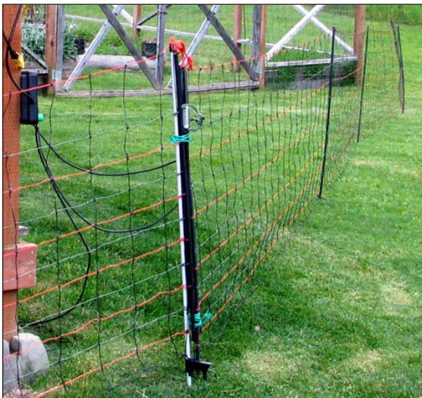
Figure 7. A premanufactured ground-return (pos/neg) electric net fence. The orange horizontal wires are electrified, and the green horizontal wires are grounded. The vertical black lines are non-conductive and secure the horizontal wires in place.
